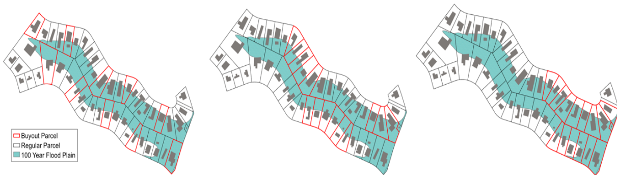
Illustration of Checkerboard vs. Contiguous Buyouts: The image on the left depicts a checkerboard buyout project in which the buyout parcels are not adjacent on continuous. The center image depicts a buyout project with small groups of contiguous parcels that are not connected to each other. The image on the right shows a contiguous buyout project in which the buyout parcels are all adjacent to one another and located within the same area. Preference will be giving to buyout projects that propose contiguous parcel buyouts like that which is shown on the right.
