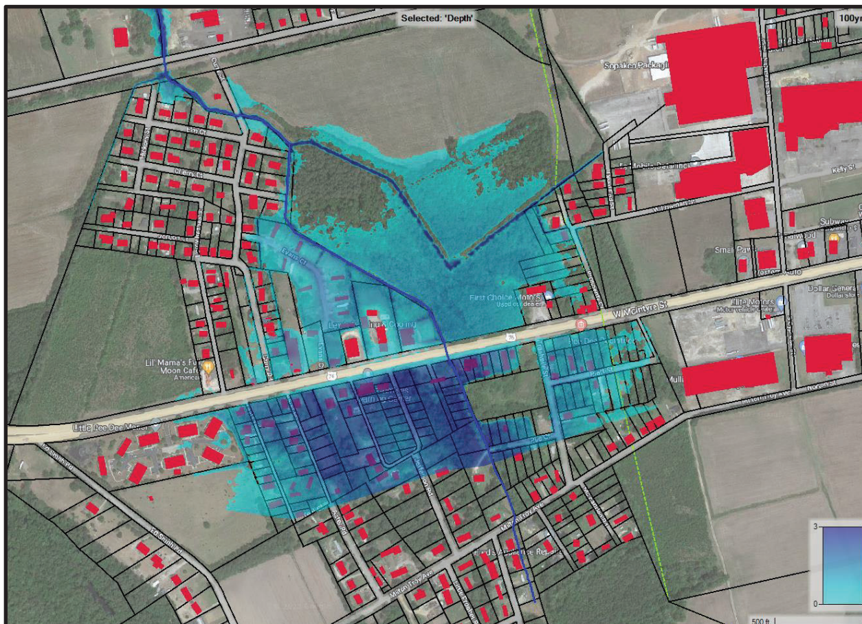
Figure 11: View of approximate existing 100-YR inundation depth upstream of West McIntyre Street (US-76).
