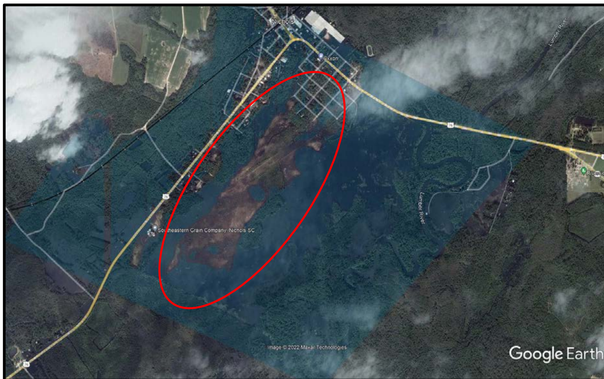
Figure M5: 100 year flood inundation from the 2D model matches very closely with actual aerial photography from Hurricane Florence (2018). The peninsula that was the site of the former airport is circled in red.
