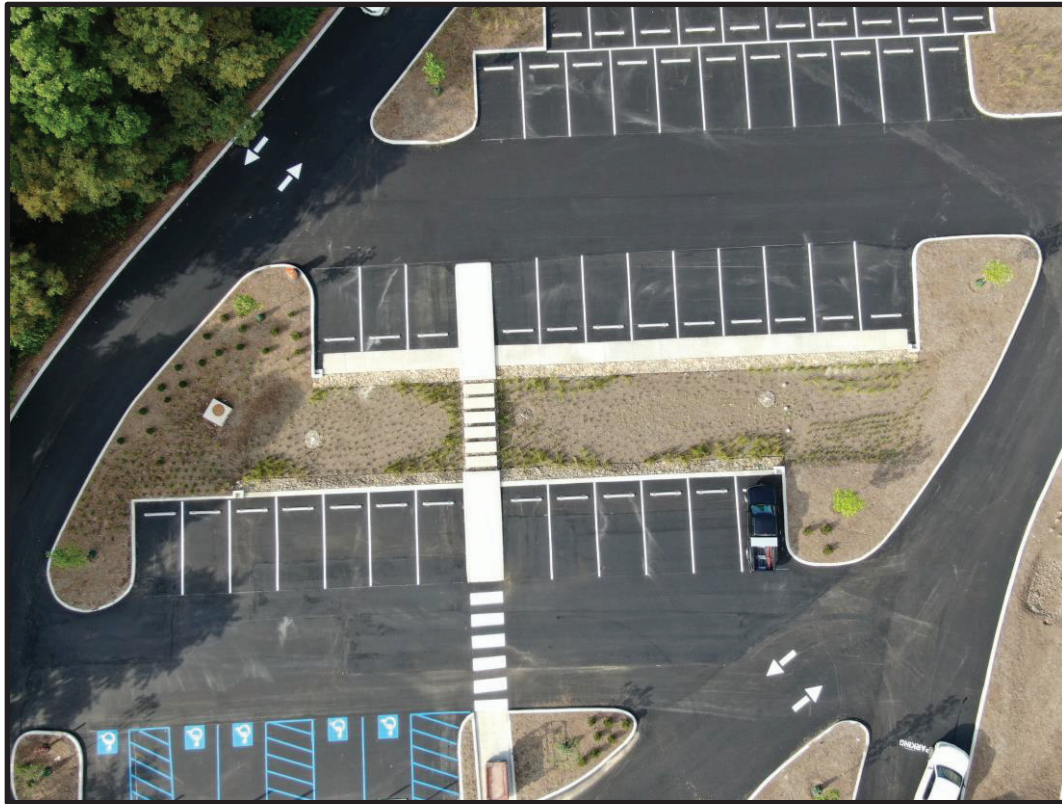
Figure O6: Aerial image of a retrofit bioretention cell designed by MBI.
