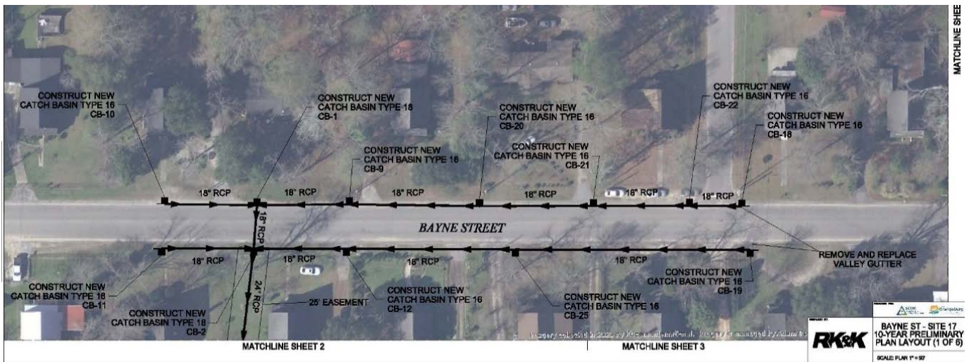
Figure 24b. Bayne Street – Proposed Improvements: Catch Basins
