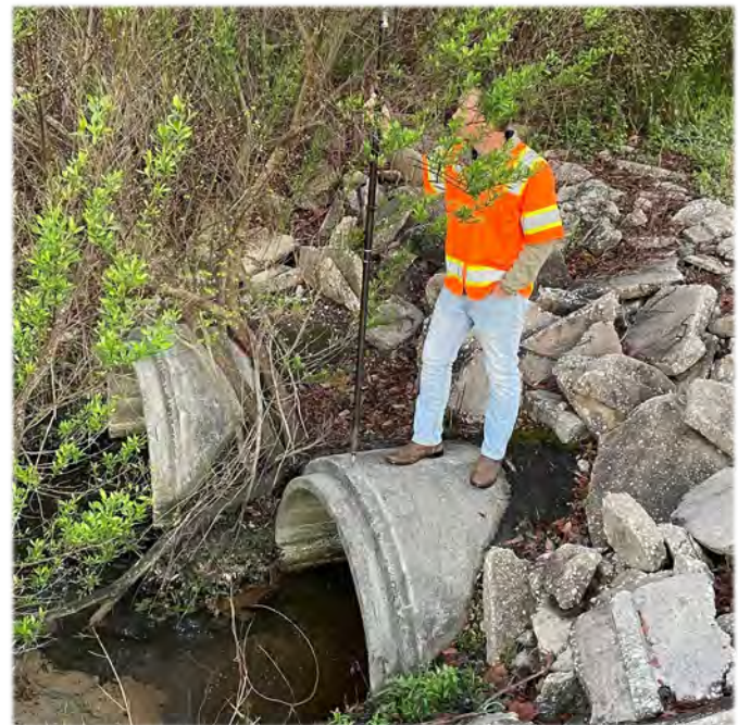
Figure 3 – Example of drainage system inventory using GPS units at outfall in the phase 1 Study Area.
