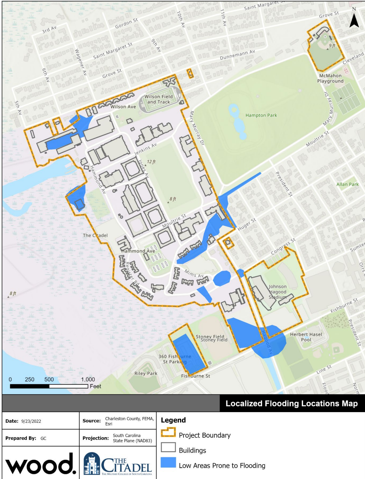
FIGURE 4.19 – AREAS OF LOCALIZED STORMWATER FLOODING
