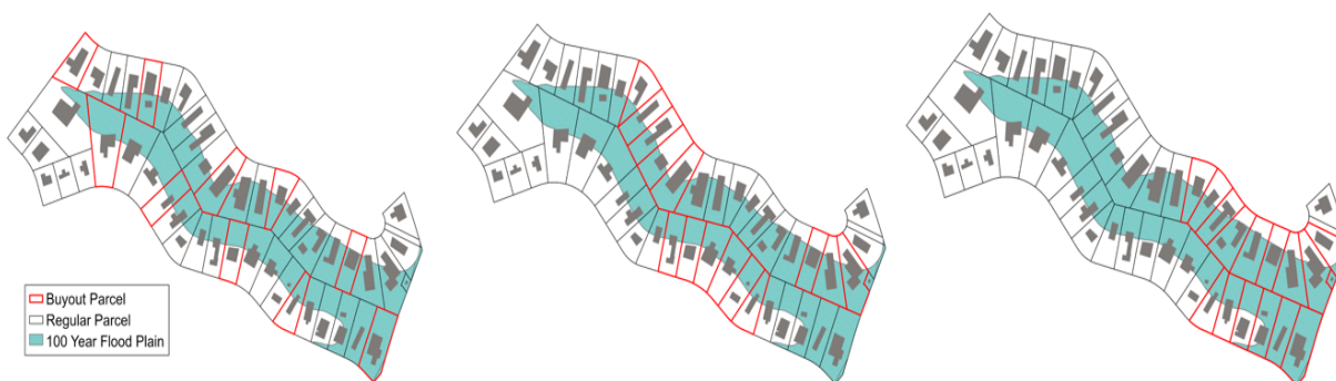
Illustration of Checkerboard vs. Contiguous Buyouts: The image on the left depicts a checkerboard buyout project in which the buyout parcels are not adjacent or continuous. The center image depicts a buyout project with small groups of contiguous parcels that are not connected to each other. The image on the right shows a contiguous buyout project in which the buyout parcels are all adjacent to one another and located within the same area. Preference will be given to buyout projects that propose contiguous parcel buyouts like that which is shown on the right.
